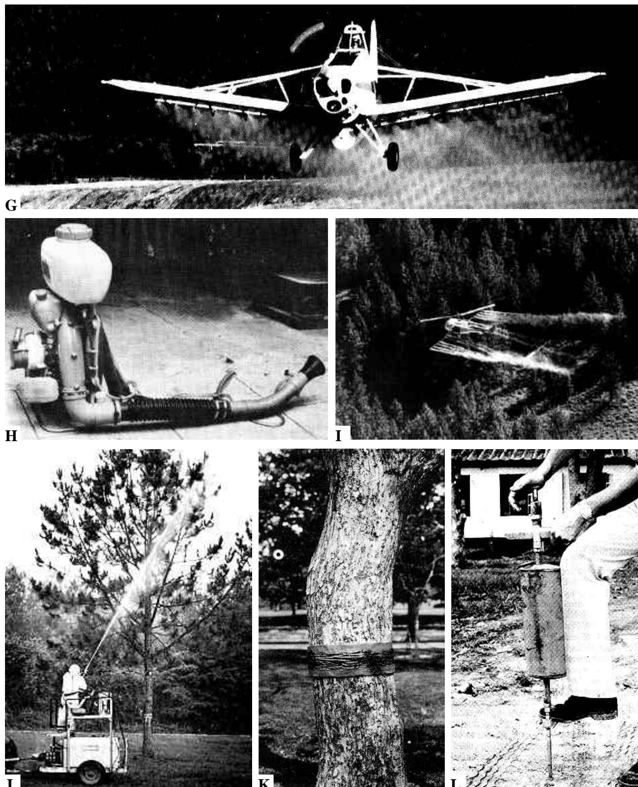
Fig. 8-19: Pesticide Applicators: (A ‡ ) ultra low volume applicator (ULVA); (B ‡ ) air blast sprayer; (C § ) lever-operated knapsack; (D ‡ ) motorised hydraulic knapsack; (E ‡ , F ‡ ) hand-held controlled droplet applicators (CDA); (G ss ) fixed wing aerial insecticide application; (H ** ) motorised knapsack mist blower; (I † ) aerial insecticide application using a helicopter; (J ** ) hydraulic insecticide sprayer; (K ss ) bait barrier preventing the descent of immature stages of pests from the crown into the soil or litter; (L +++ ) soil applicator (reproduced from Queensland DPI, 1990 ‡ ; DAL, 1986 § ; Hill, D.S. and Waller, J.M., 1982 ** ; Ross, H.H., 1982 ss ; Barbosa, P. and Wagner, M.R., 1989 † ; Coulson, R.N. and Witter, J.A., 1984 ** ; ICI +++ )
